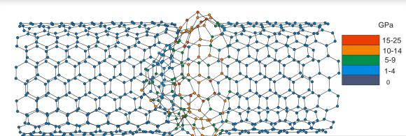
Destruction of the structure of bamboo-like CNT during the increase of the temperature
