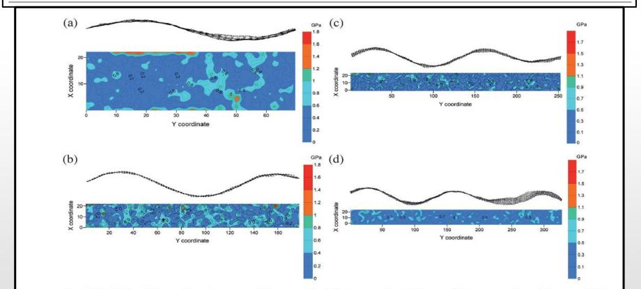
Map of distribution of the local stress for the nanoribbon armchair: (a) in the case of two half-waves; (b) in the case of three half-waves; (c) in the case of four half-waves; (d) in the case of five half-waves.
