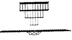
The deflection of the graphene sheet (620 atoms) by means of the platinum pyramid (376 atoms).
