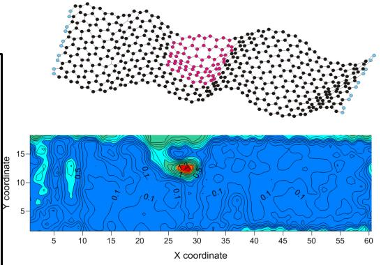
Defects of the C–C bond are observed only between atoms with a local stress value of about 1.8 GPa. One of the most stressed sections of the atomic grid containing a defect is presented in Fig. 4. From the Figure it is clearly seen that after C–C-bond breaking the atomic grid reconstructs and the stress decreases. The enthalpy of the defect formation equals  $163.5 \text{ kcal mol}^{-1}$ . GPa
